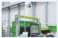
Hand camera used to check work procedures by workers
