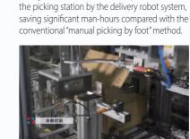
Automatic insertion of delivery slip Delivery slips are automatically inserted into shipping boxes. Full automation from printing delivery slips to inserting them into boxes minimizes a risk of erroneous insertion
